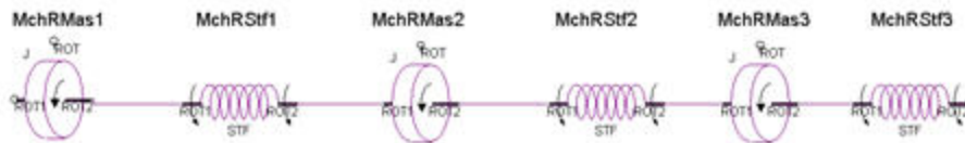
Figure 3. The rotational four-body system model in Twin Builder
